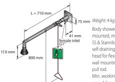
Body shower, wall mounted, modular in SS & Stanniloy with self-draining shower head for flexible wall mounting with pull rod. Min. working pressure: 1 bar.
