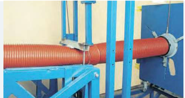
Stress test: 100% tightness with 30% deformation
